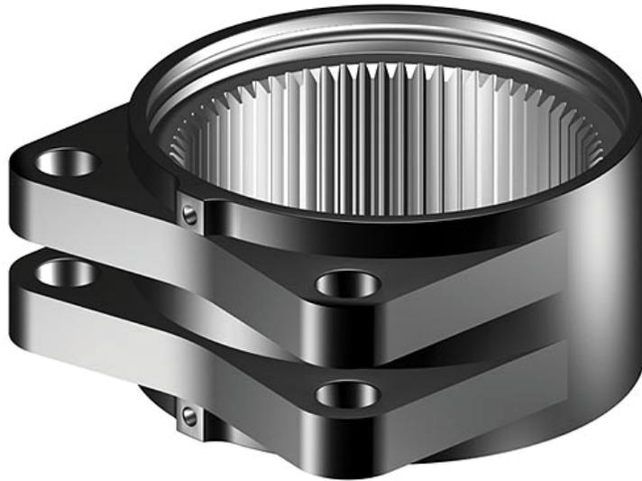
Large significant technical illustrations may require more than two line weights to accurately depict spatial relationships. When using five lineweight rendering, you must make a careful analysis of the function of each line on the object and an initial decision as to the position of the sun. The sun's position determines which exterior lines are the heaviest as well as the position of any highlights.
