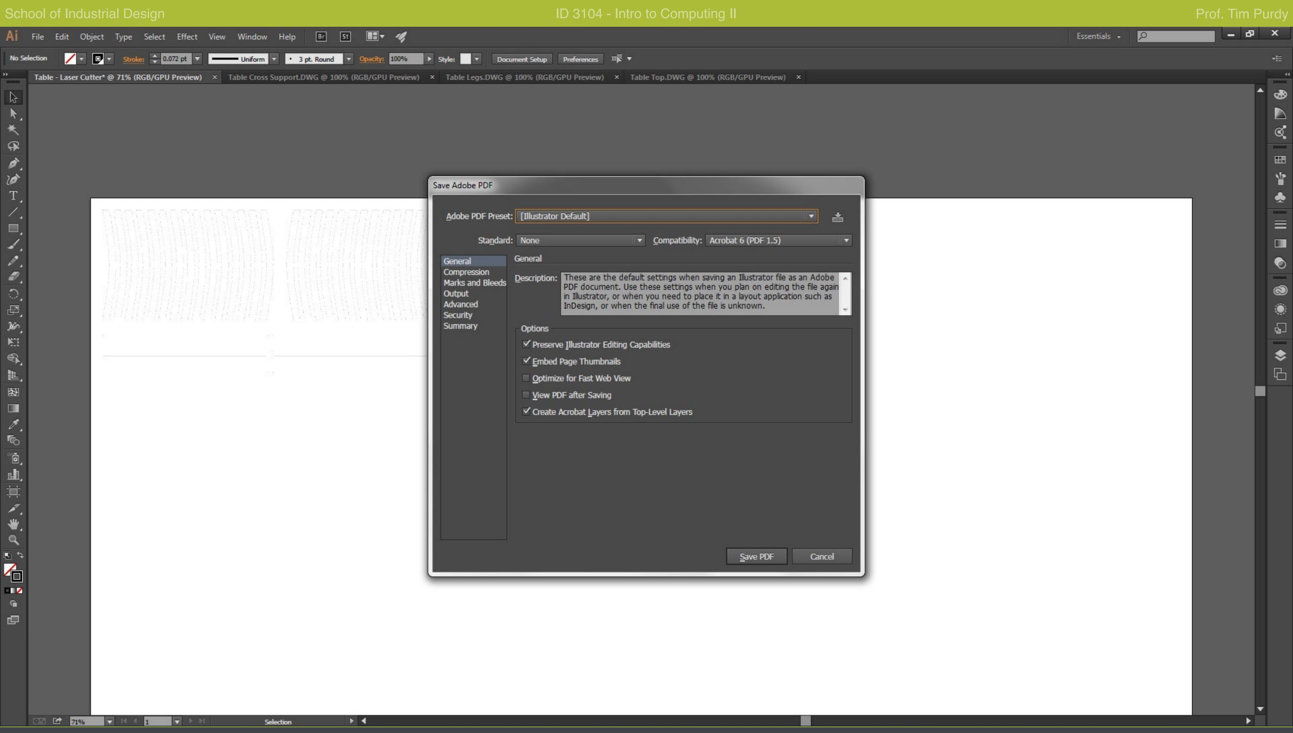
Save the file as a PDF using the Illustrator Default option. Use the PDF file to print in the laser cutters.
