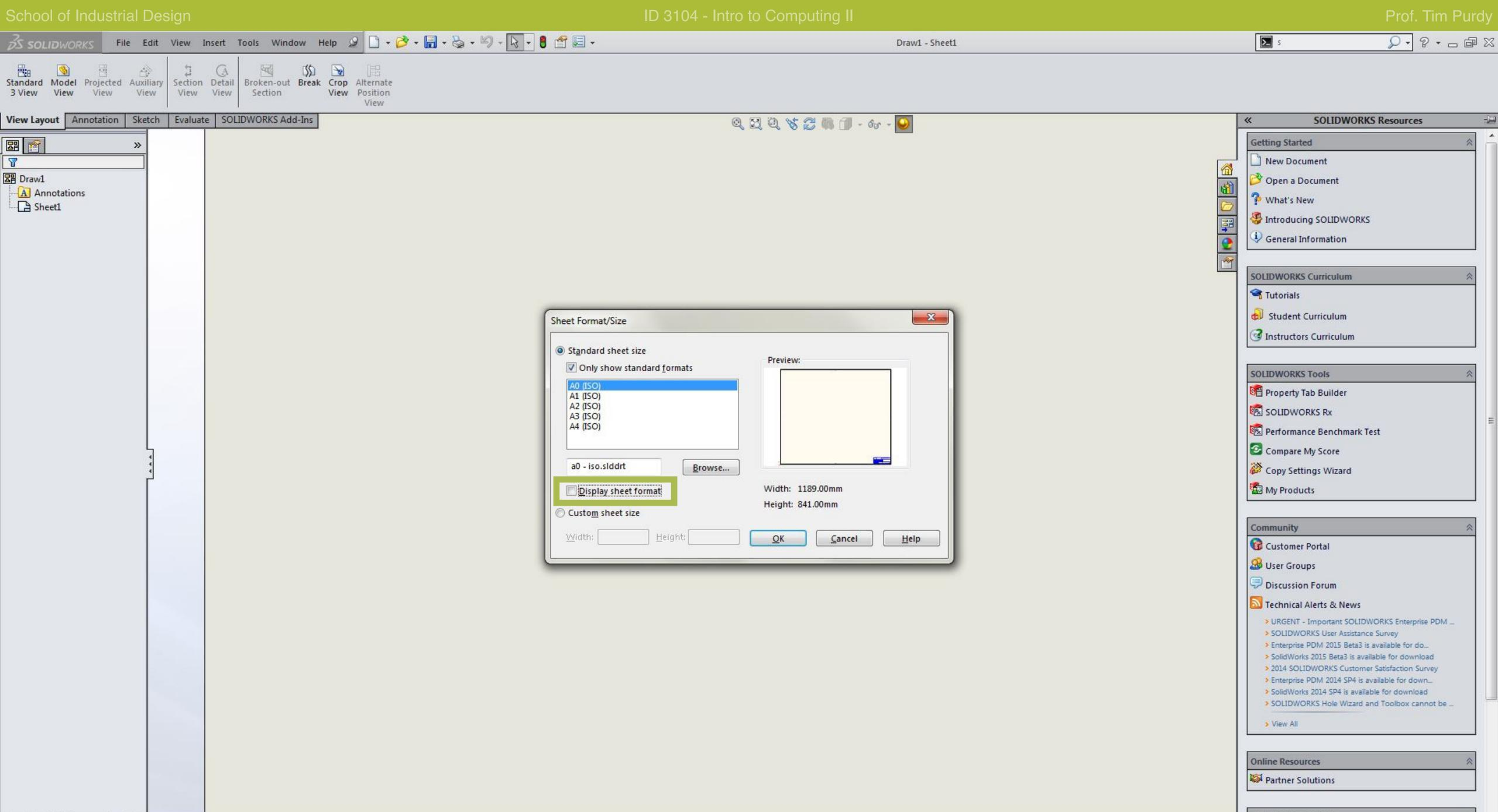
In the Sheet Format/Size dialog, uncheck the Display Sheet format box. The sheet size doesn't not matter since we are going house only the drawing.
