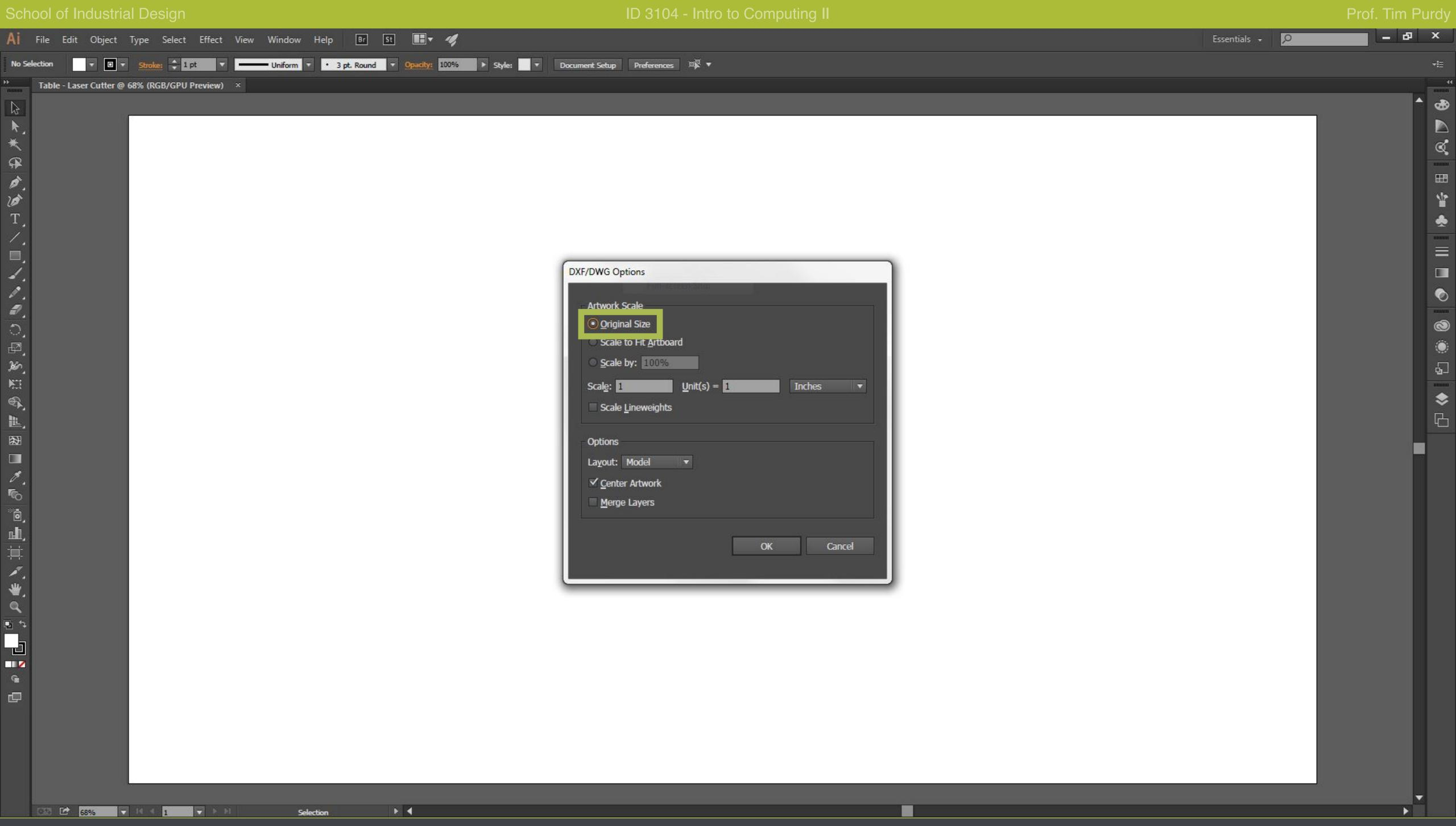
In the DXF/DWG Options box, choose the Original Size option. This avoids any scaling since the drawing is already scaled to 1:10.
