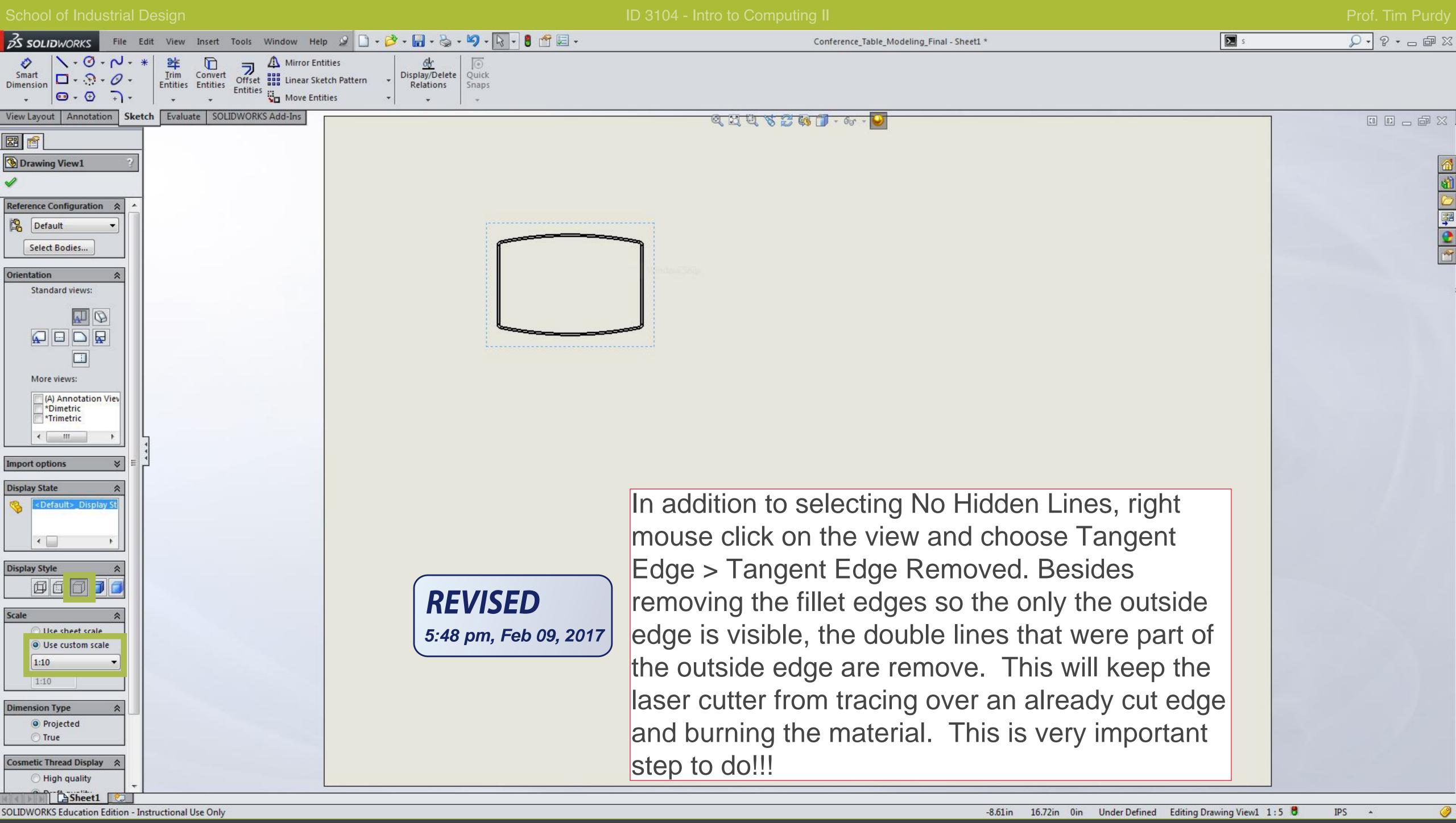
Press Esc to cancel the insert command and click on the drawing to select it and bring up the options in the sidebar. Ensure that the Display Style is set to No Hidden Lines (third option). Coosing any other option creates overlapping lines which may cause issues when cutting the file in the laser cutter. Set the scale to 1:10 from the list.
