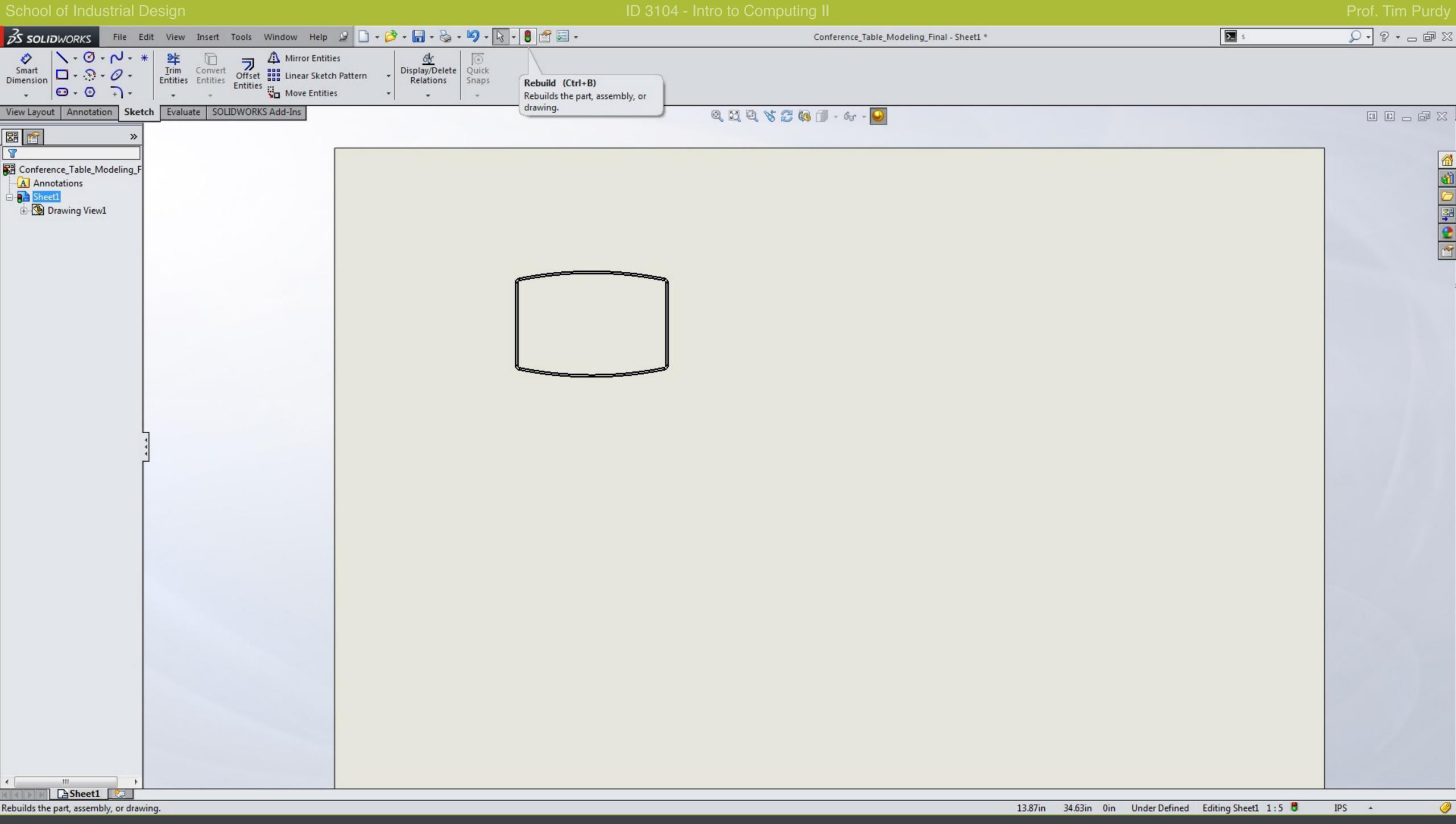
Use the Window menu to switch back to the Drawing window. Click the Rebuild icon in the Menu Bar to refresh the drawing file.
