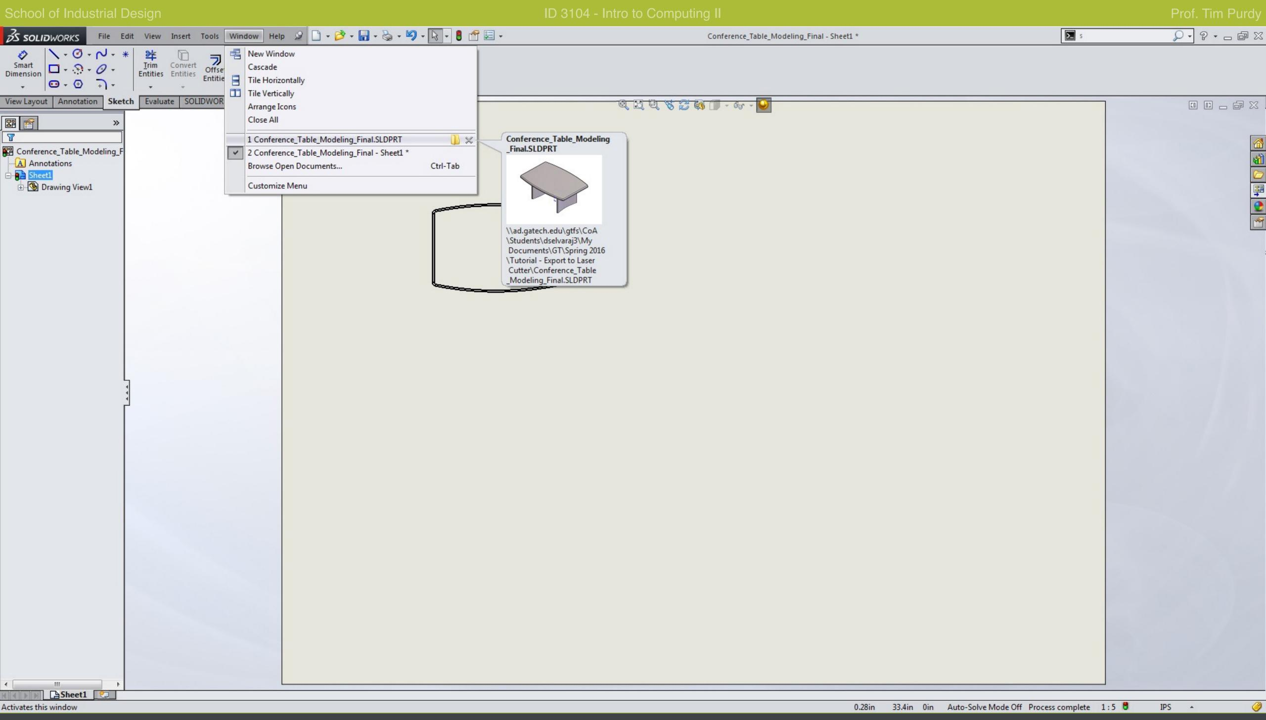
Switch back to the model window by selecting it from the Window menu in SolidWorks.
