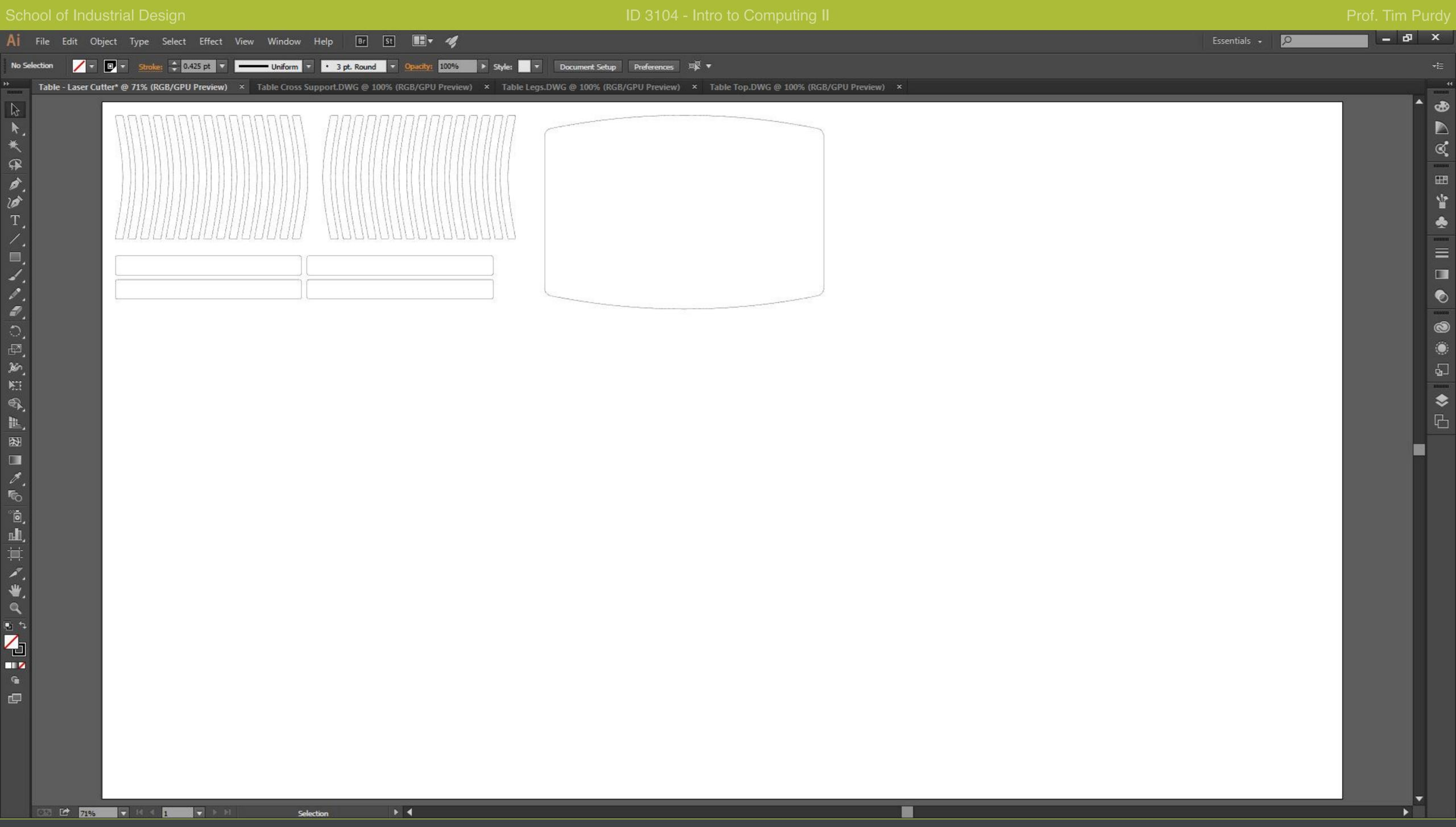
Make copies and lay it out to fit the area of the material you will be using to cut.
