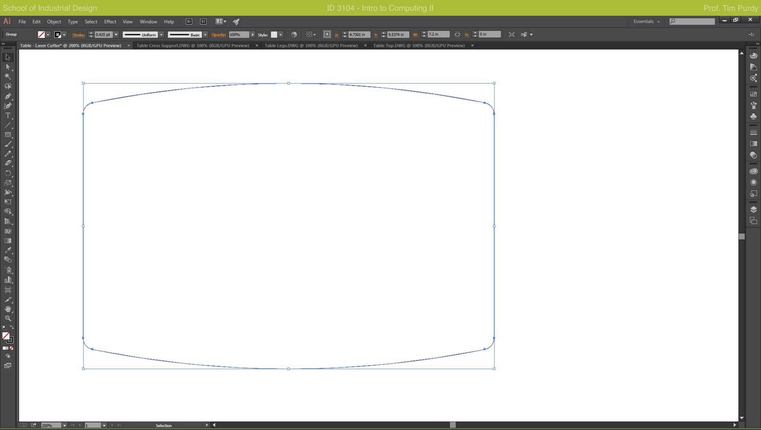
Select all the pieces of the loop and press Ctrl + J (Cmd + J on a Mac) to join all the pieces to form one complete loop.
