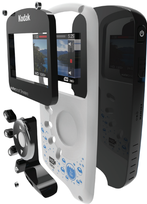
Figure 1 - Each color area was modeled as a separate solid.
