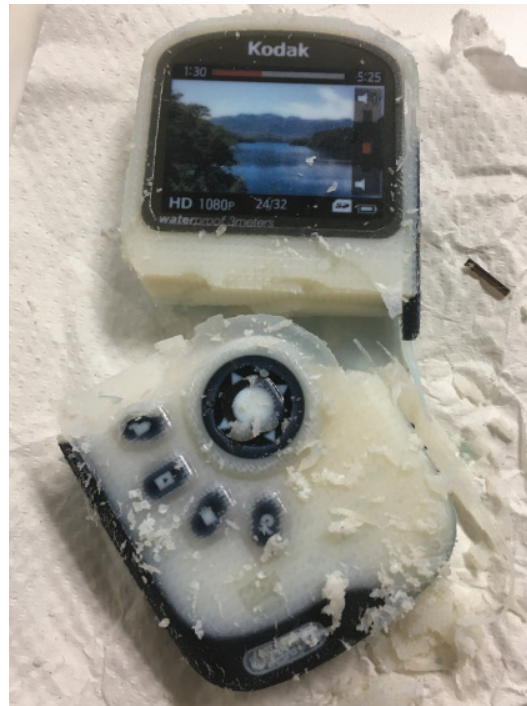
Figure 2 - Failed print, form was mostly a shell with internal support material
