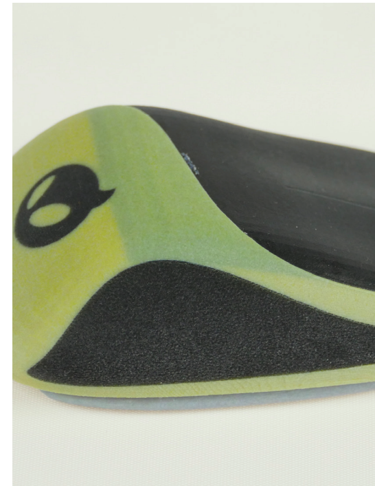
Figure 3 - A solid shell with bottom open to allow supports to be removed
