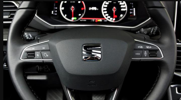
The left part of the multifunction steering wheel in terms of functions and icons is similar to that of the Seat Tarraco. Above all, the buttons to control the individual areas in the Instrument Cluster, the view button and the scroll wheel for navigating through the individual content of the Instrument Cluster are clearly recognisable.
