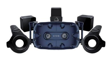
The Vive Pro Headset is blue with no rings around the front cameras. It has a resolution of 1440 x 1600 per eye, 90Hz max screen refresh rate and 110° field of view.
